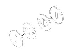
**2.** Fit key escutcheon plates with the screws provided.
